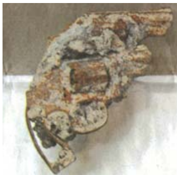
INTENSE HEAT: Two handguns, believed to be .357 Smith and Wesson models that were stored in federal offices in the World Trade Center, were found forged together, an indication of the intense heat from fires started on Sept. 11.
